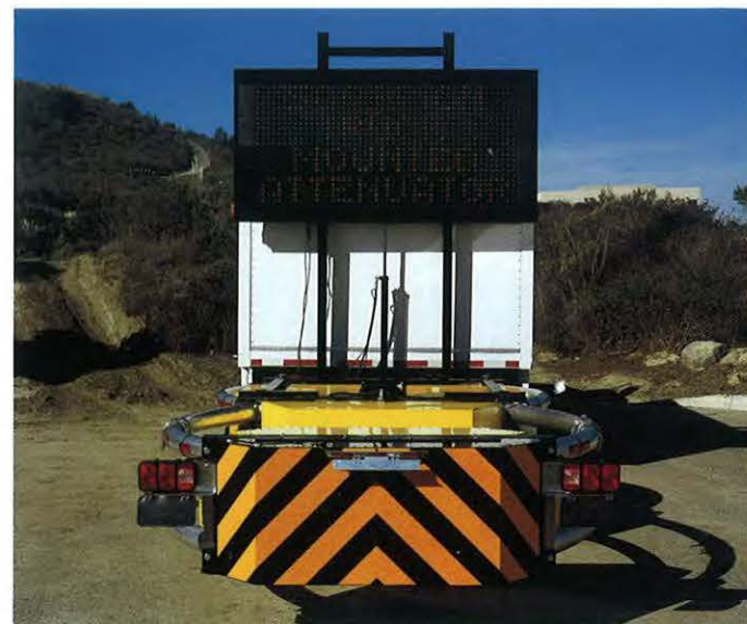
Rear view of the Scorpion TMA with message panel in the raised position, ready for use on the job site. The bottom of the message panel when elevated, is 7' above the surface of the roadway, in full compliance with Federal Standards.
