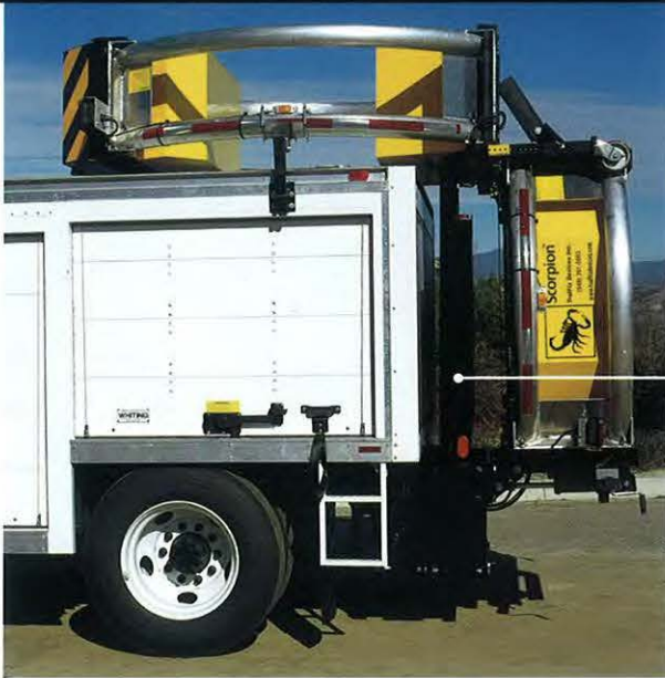
The Scorpion TMA and message panel in the storage or transport position.
