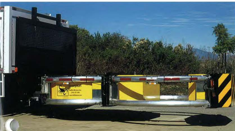
The Scorpion TMA is fully extended, with the changeable message panel in the travel or storage position.
